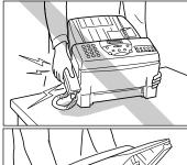
• If you have installed the optional handset, do not lift the fax by the handset cradle.
